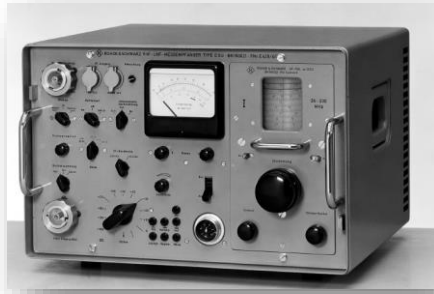
ESU VHF/UHF frequency range from 25 MHz to 900 MHz
